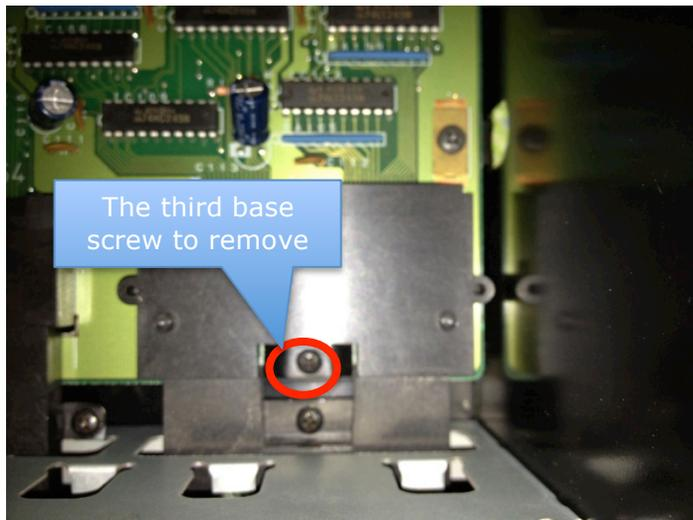
With all the screws removed, the front should now be easily removed. As you move it forward, it needs to drop down as well to clear things.
