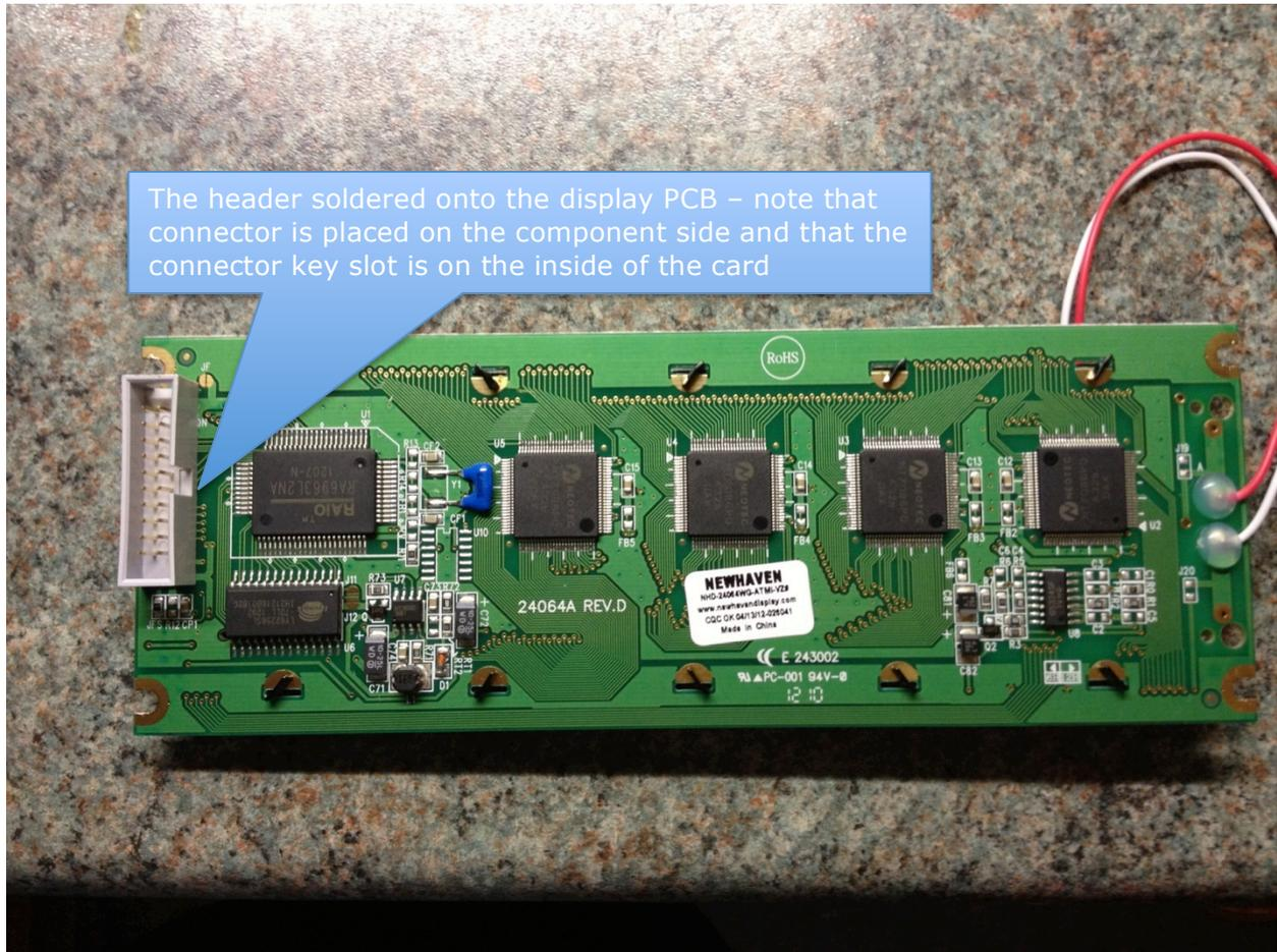
Note that the connector goes on the component side of the card, like the directly soldered connector on the display that you have just removed, and the key slot faces towards the components.
