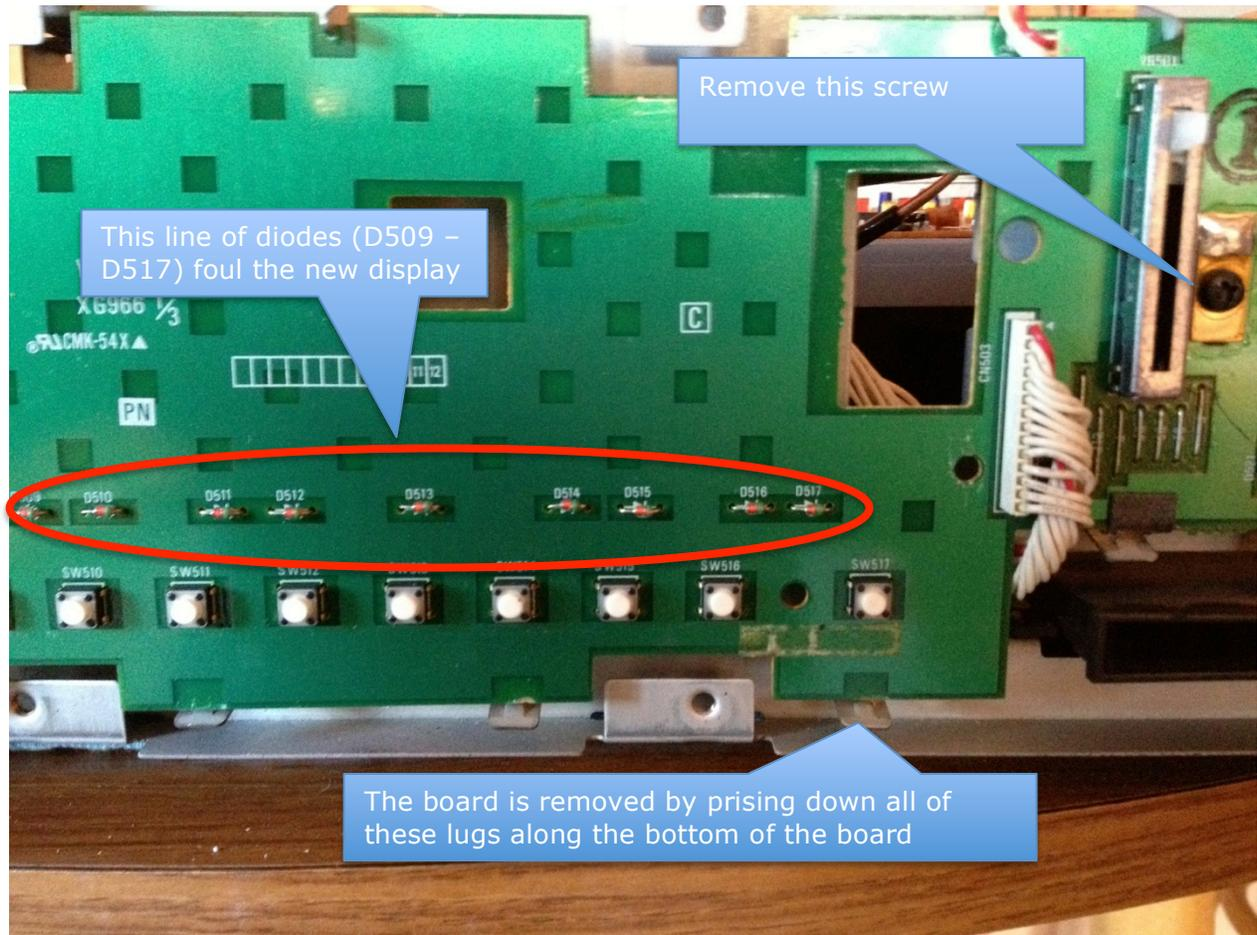
You need to prise down all of the lugs that hold the board at the bottom. There is also a single screw by the Data Entry slider.
