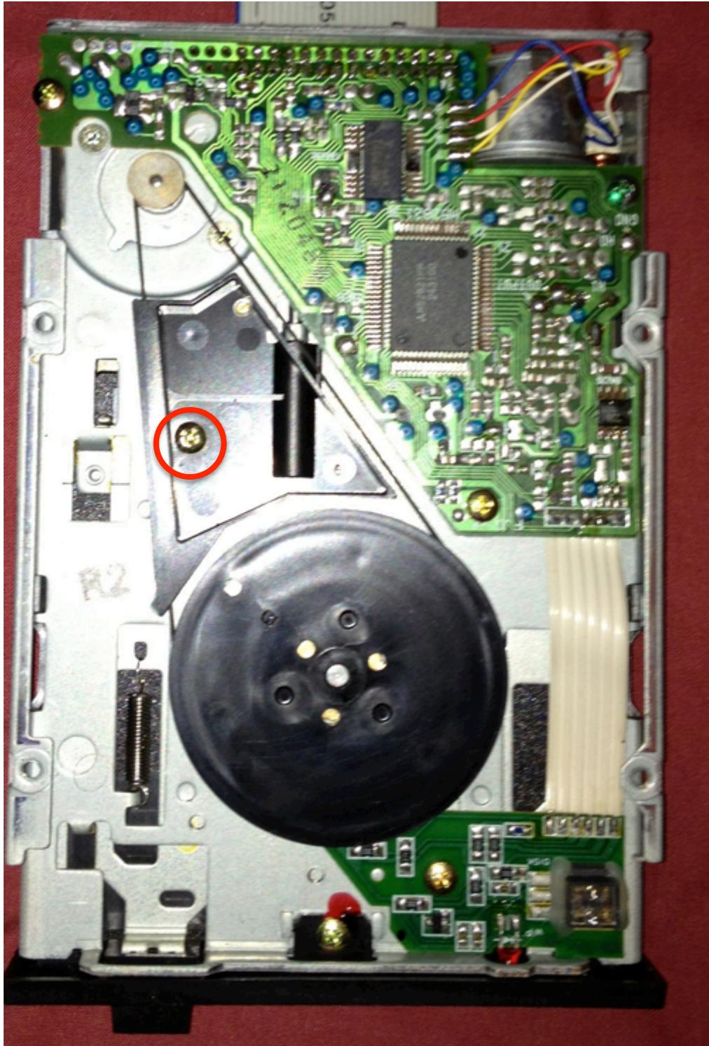
Once this screw is removed, the belt guard lifts off, and you can now remove the old belt and fit the new one.
