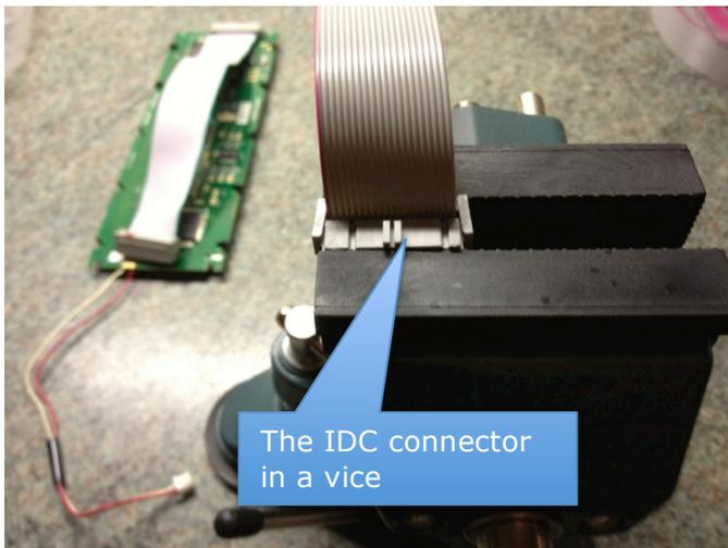
Note that you need to get the orientation of the plugs on the cable correct, to match the connector keys either end. Use the existing display (in the foreground in the picture below) to get this right.
