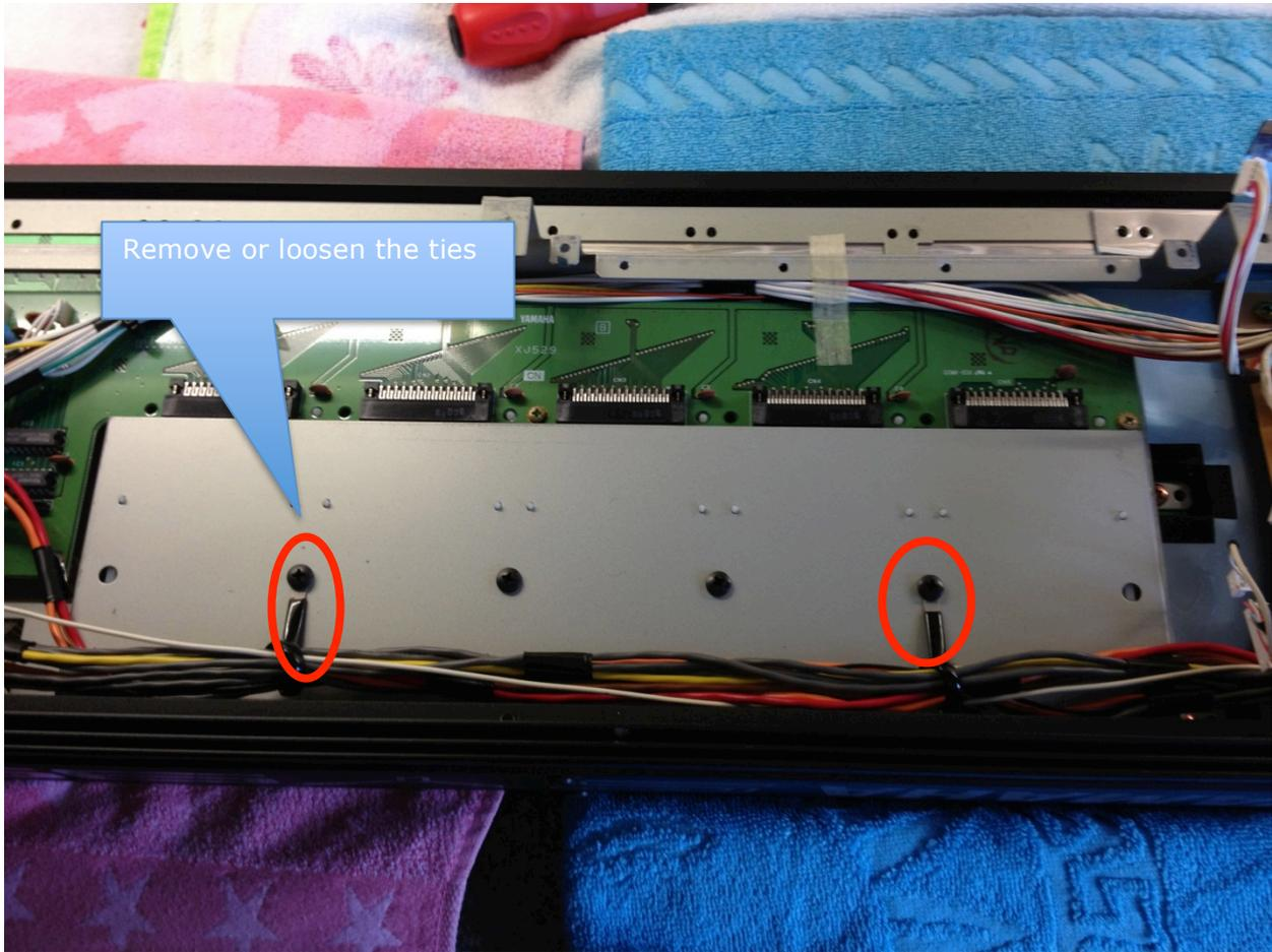
Undo the screws holding the sample RAM chassis. There are two recessed screws either side of the chassis.
