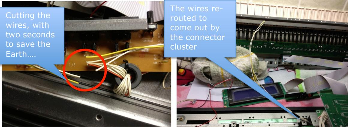
As mentioned, earlier, this 5V supply is outside the quoted range of the new Display's LED backlight, so we need to simply drop some voltage. This is done by putting a resistor in series with the negative line of the supply. Again, I elected to use a 1K trimmer rather than experimenting to find the right value.
