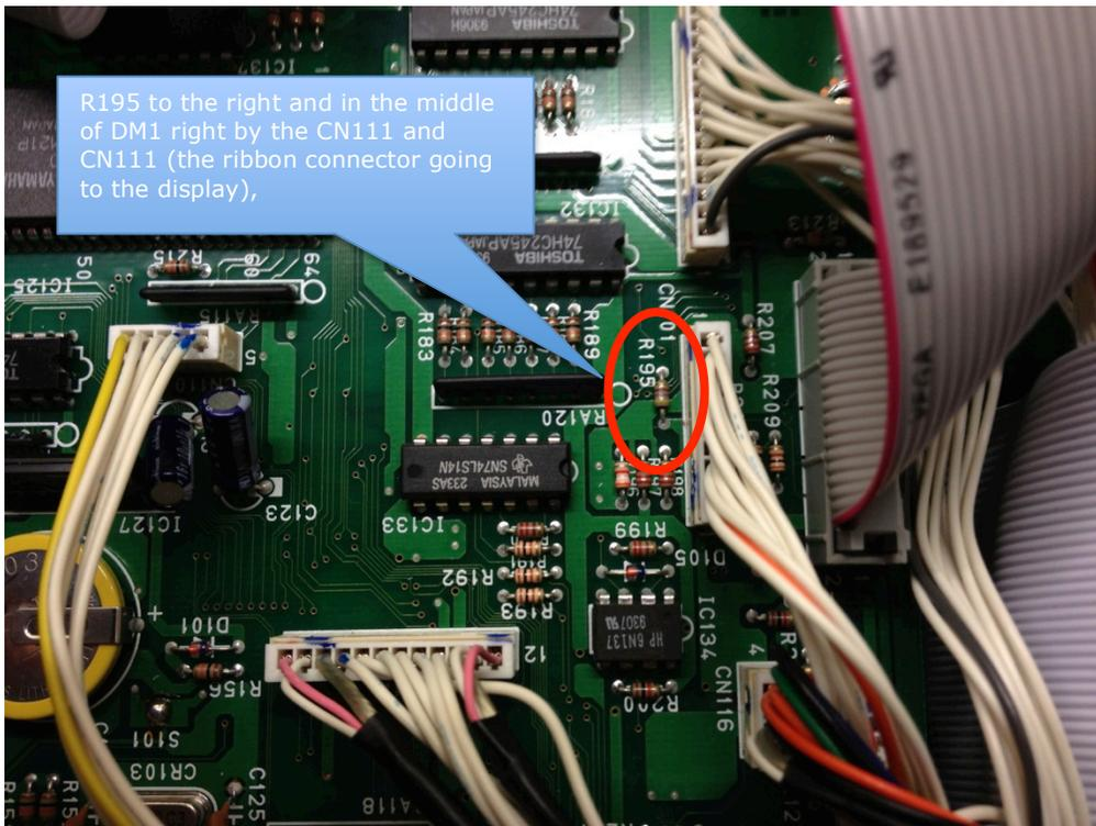
Rather than try different resistor values (and so need a whole load of resistors!), I elected to use a multi-turn trimmer (variable resistor) with a value of 10K. I snipped the 3<sup>rd</sup> leg off and formed the other two to fit the lead spacing of R195.
