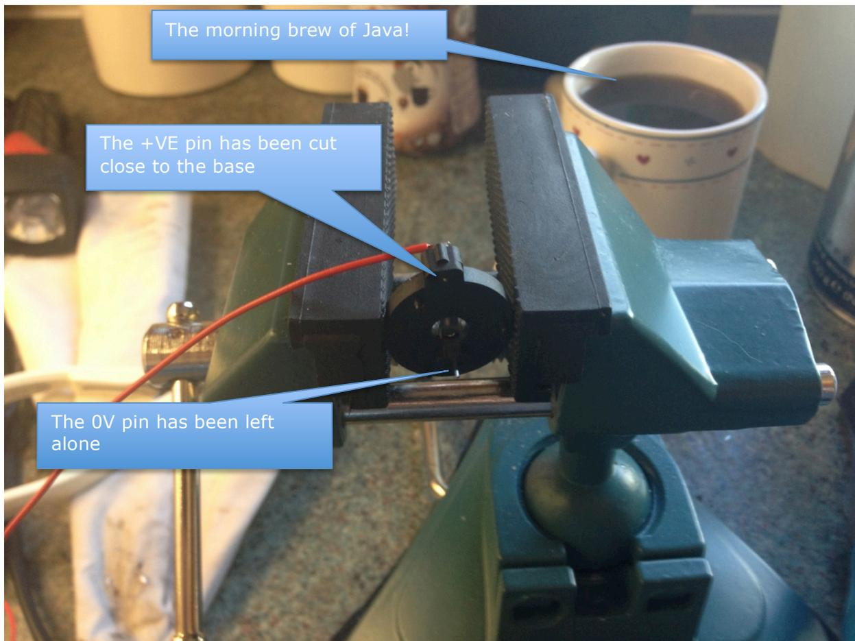
Solder a lead direct to the +VE terminal on the top of the holder.
