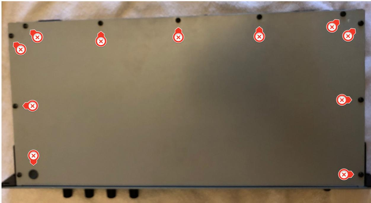
Now you can remove the case, and you will have the following view. The front of the FS1R is towards the bottom of the picture.
