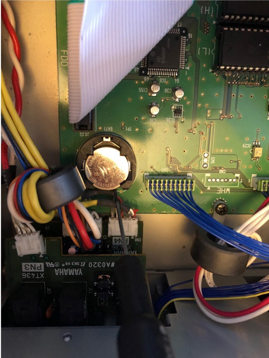
Now the old battery is removed, quickly insert the new battery, with the text CR2032 facing upwards. It should slide into place quite easily as you push it in from towards the front of the synth towards the back.
