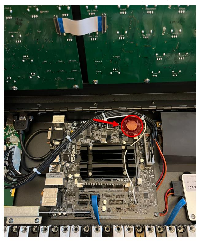
Before removing the battery, ensure that the other one is ready. Some batteries now come with a self-adhesive warning sticker that needs removing first, so you want to remove that if present, otherwise the circuit will not be made!
