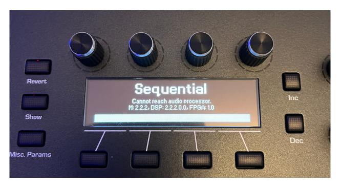
The general experience on the internet forums is that is usually due to either marginal power supply voltages or a dead CR20232 battery, so the first step was to see if the battery needed replacing.
